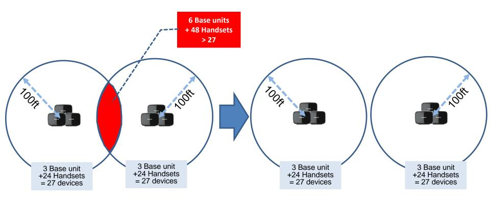
If there are adjacent areas of such Very High Density, each area should not be overlapped each other to keep the total number of devices in this overlapped less than the limit, i.e. not exceed 27 (15 in wideband mode).
