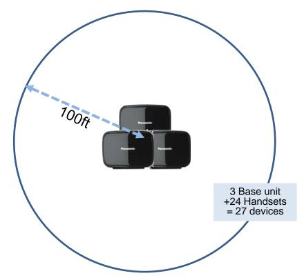
If Very High Density in one area with 100ft radius is needed, the maximum 3 Base units can be placed near the center of the area. In this case, the individual Base unit should be at least 2ft apart from each other.
