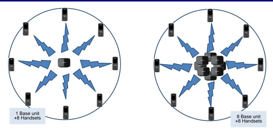
Only one KX-TGP600 Base unit is necessary to support 8 (4 in wideband mode) simultaneous calls within a range of 100ft radius as left figure.
