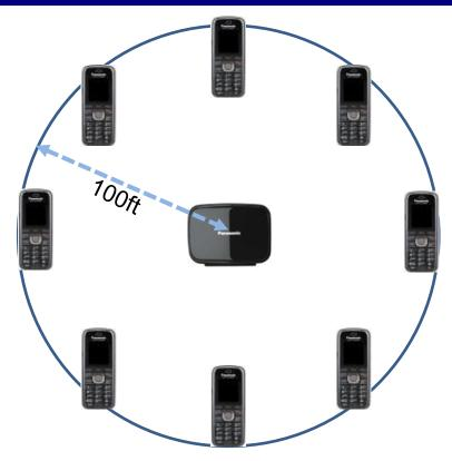
One KX-TGP600 Base unit can support 8 (4 in wideband mode) Registered Handsets and 8 (4 in wideband mode) Simultaneous calls within a range of 100ft radius in a standard indoor environment.
