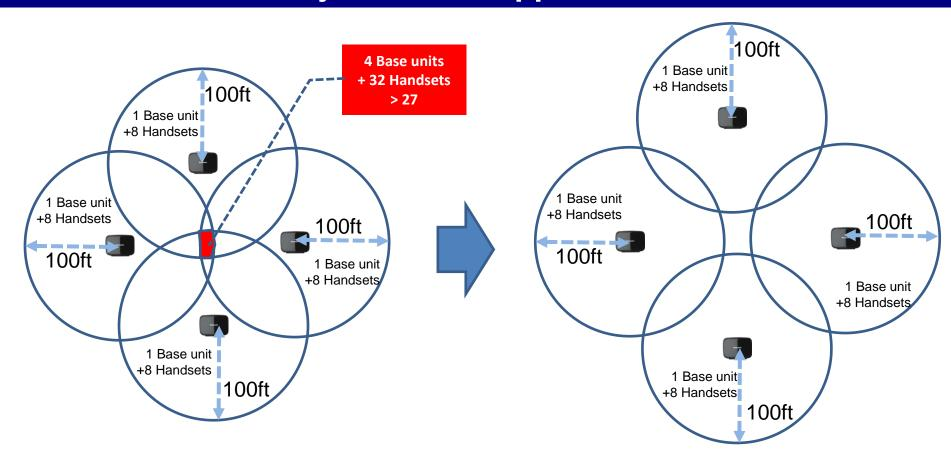
If many areas of 100ft radius around the Base unit are overlapped, the total number of devices in this overlapped area may exceed 27 (15 in wideband mode). In this case, the distance between Base units should be longer each other to avoid too much devices.
