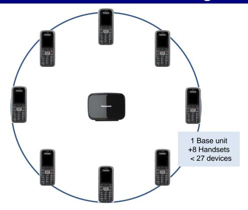
When you install multiple Base unit, you should consider the Total Number of Devices (Handsets and Base units) within a range of 100ft radius.
